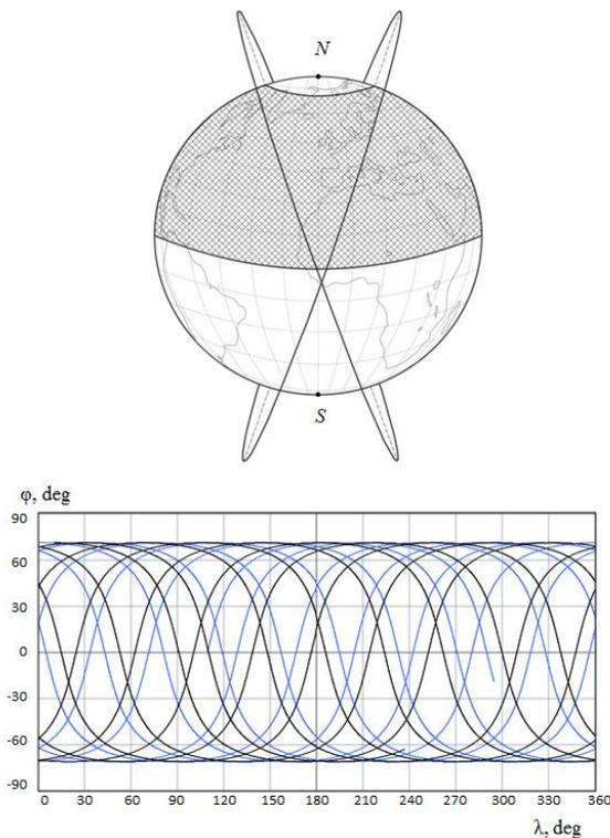
**Figure 1. Traditional two-satellite constellation and a corresponding ground-track ( $H = 3000$  km,  $i = 71^\circ$ )**
