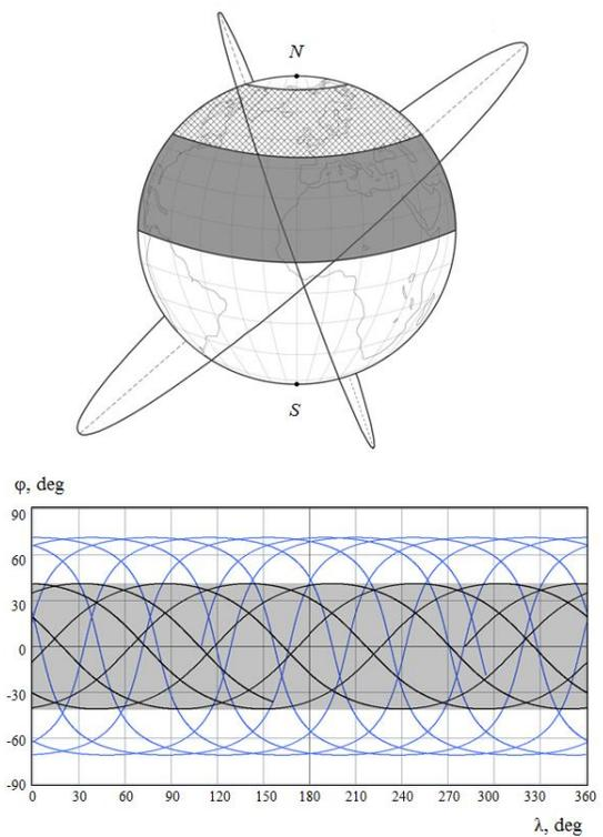
**Figure 2. Compound two-satellite constellation incorporating two NR-synchronized orbits and a corresponding ground-track ( $H_1 = 3000$  km,  $i_1 = 71^\circ$ ,  $H_2 = 5545$  km;  $i = 41^\circ$ )**
