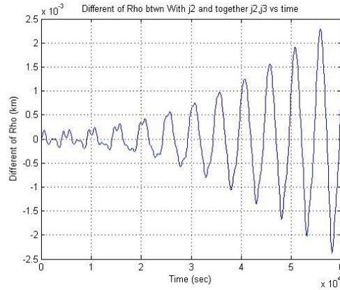
Figure 8 The difference in the radius of the orbit of the Deputy Satellite around the Chief Satellite between the solution of J2LMCW and the solution of J3LMCW.
