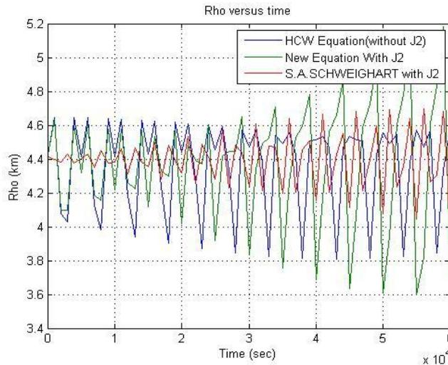
Figure 7: Comparison of the Deputy Satellite orbital radius around the Chief Satellite as the solution of the baseline Clohessy-Wiltshire Equations, the linearized  $J_2$  modified HCW Equations and similar solution obtained by Schweighart [17].
