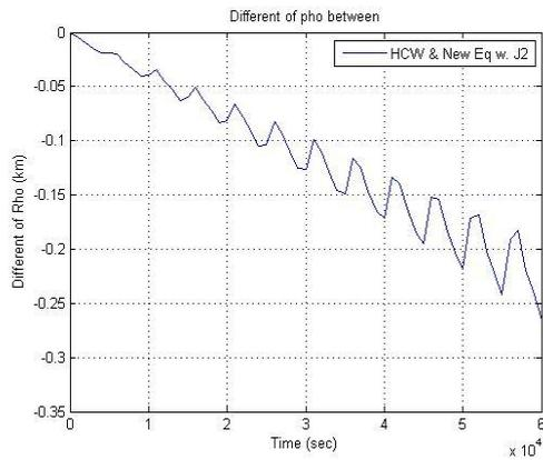
Figure 4. The difference between the radius of the orbit of the Deputy Satellite around the Chief Satellite as the solution of the original linearized HCW Equation (without  $J_2$ ) and that incorporating the influence of  $J_2$ , using linearized  $J_2$  modified HCW Equation
