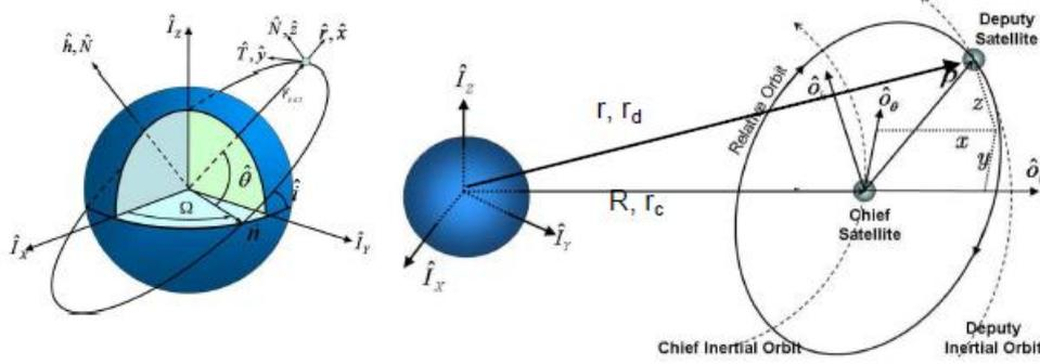
Figure 1. The  $(r-\theta-i)$  coordinate system is used in describing the  $J_2$  disturbance in the local  $(x-y-z)$  coordinate system.
