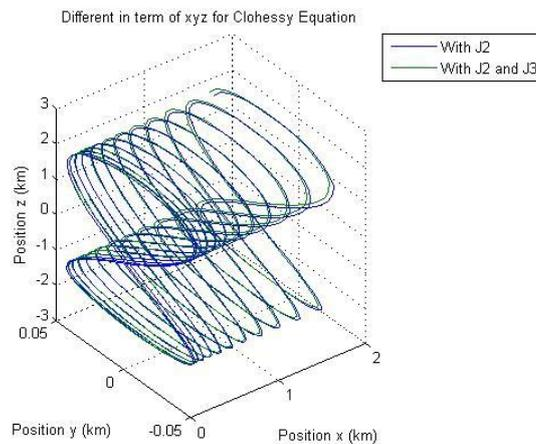
Figure 10. Comparison of the difference in the distance of the path of Deputy Satellite around the Chief Satellite in LVLH coordinate between the solution of CW Equation with J2LMCW equation and CW Equation with J3LMCW equation
