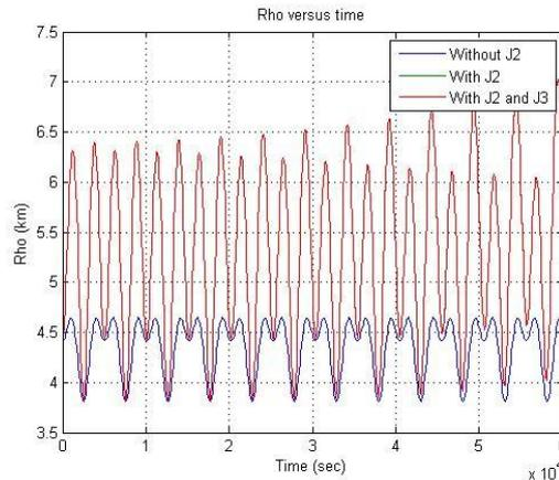
Figure 9. Comparison of the radius of the orbit of the Deputy Satellite around the Chief Satellite as the solution of CW, J2LMCW and J3LMCW.
