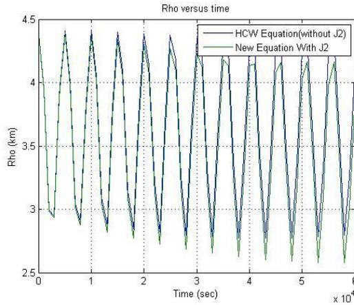
Figure 3. Comparison of the Deputy Satellite orbital radius around the Chief Satellite as the solution of Clohessy-Wiltshire Equation (without  $J_2$ ) and incorporating the influence of  $J_2$ , using linearized modified Clohessy-Wiltshire Equation.
