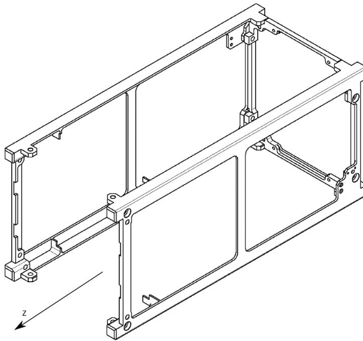
**Figure 5. 2U mechanical structure for a CubeSat (credit: M. Urbanowicz)**
