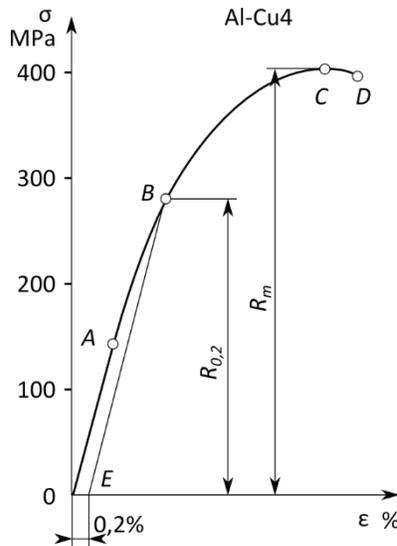
**Figure 2. Tension of an aluminum rod**
