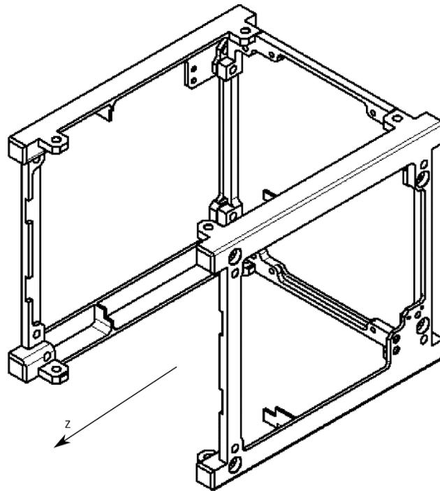
**Figure 4. 1U mechanical structure for a CubeSat (credit: M. Urbanowicz)**
