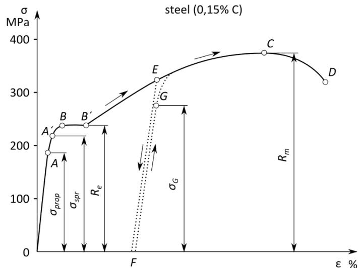
**Figure 1. Tension of a steel rod**
