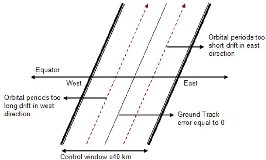
**Figure 2. Ground track drift measured at the equator.**
