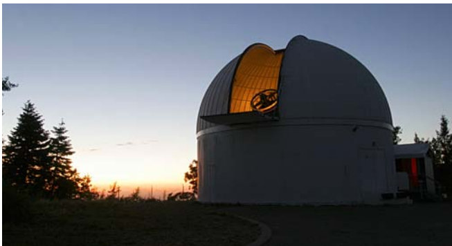
Figure 1: 1.52-meter (60") Cassegrain reflector f/2 prime focus has a 1^\circ field-of-view, detecting down to 22^{\text{nd}} magnitude objects. Located atop Mt. Lemmon, this telescope (G96) is one of three co-located ground-based facilities that comprise the Catalina Sky Survey. G96 is also used for astrometric follow-up and physical observations NEOs (University of Arizona, CSS).
