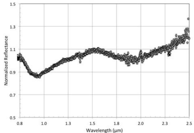
**Figure 3:** Near-IR spectrum of 2014 WC201 showing weak absorption bands at 1- and 2- $\mu\text{m}$  due to the minerals olivine and pyroxene. The scatter at 1.4 and 1.9  $\mu\text{m}$  is due to incomplete correction of telluric bands.
