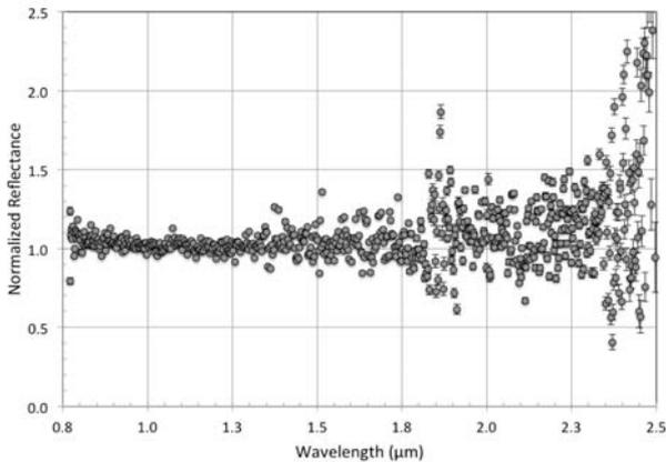
**Figure 4:** Near-IR spectrum of 2014 UV210 a rise in reflectance beyond 2.3 μm due to the shorter wavelength end of the Planck curve being shifted to near-IR wavelengths. This would suggest that the object has a relatively low albedo (<0.10). The asteroid was at V magnitude 18.7 at the time of observations.
