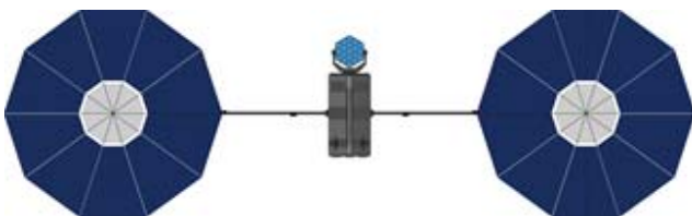
Figure 3. Conceptual design of the deployed spacecraft with two 15 m PV arrays that produce 50 kW each at the beginning of life for a total of 100 kW electrical, ion engines at the back, and the laser array pointed directly at the viewer. A 2 m diameter laser phased array is shown with 19 elements, each of
