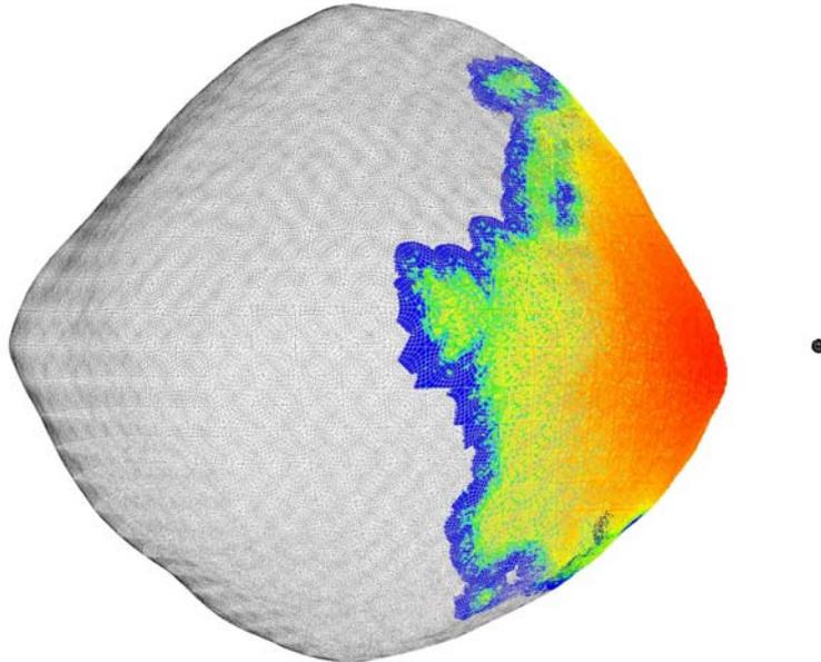
**Figure 1 -- Surface material velocity on a 3D model of Bennu (a 493 m diameter NEO) 400  $\mu$ sec after exposure to a 1 Mt standoff nuclear detonation. The small sphere to the right of Bennu indicates the position of the energy source, roughly 100m above the equator. The color scale is logarithmic in velocity: blue is material moving less than 30 cm/sec, while the peak in red is expanding at 20 km/sec.**
