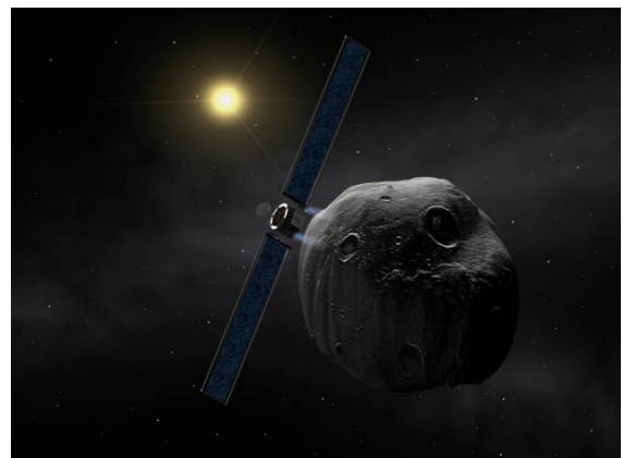
Figure 1: The gravity tractor as currently envisioned. Top: Overall configuration. The S/C is built around an ESPA ring main structure and features 4 pods of SEP based RCS thrusters canted at an angle \beta = 45^\circ . The RCS thrusters are responsible for both attitude control and the translational hovering with respect to the asteroid. Bottom: impression of the gravity tractor during the hovering phase close to the asteroid.
