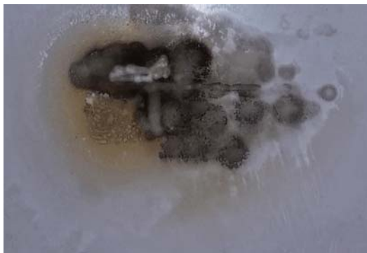
Figure 12. Laboratory experiment quartz blast shield that has undergone multiple ablation measurements. The ring of brown debris shows basalt sample ejecta from recent measurement. The black shows ejecta from the multiple laser ablation measurements embedded in the quartz.
