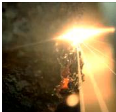
Figure 9. Right photo was taken during a low pressure ablation test and shows mass ejecta and plume. Left photo was taken during an ablation test at ambient pressure and shows the sample smoking and melting.
