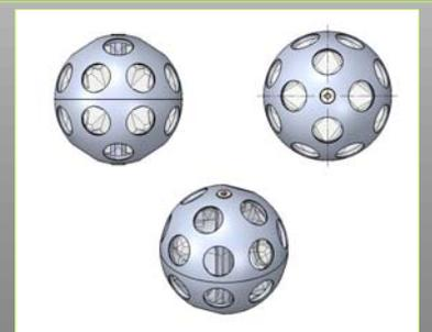
INRRI-S LRA, equipped with twenty four CCRs. Diameter is about 2 inches; total mass is about 65gr
