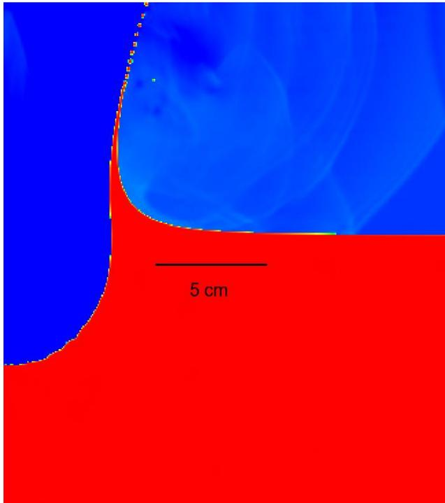
*Figure 1: Crater in PAGOSA simulation at 300 microseconds.*
