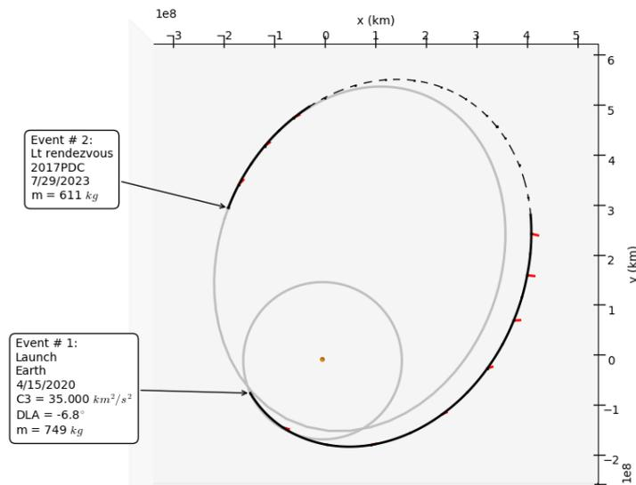
**Figure 3: Low-thrust trajectory for a rendezvous observer arriving at 2017 PDC on July 29, 2023.**
