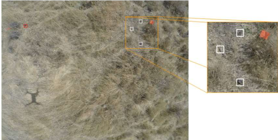
Figure 3: Sample output from the bag of convolutional neural network classification algorithms where the input is an image taken by the UAV. Red boxes are drawn over patches which output 0.75 or higher, and white boxes are drawn over patches with output 0.5 to 0.75. The orange flag in the image marks where the 2 meteorites were placed, both of which were detected in the white boxes. Only 2 boxes are incorrectly labeled out of about 60,000 boxes examined.
