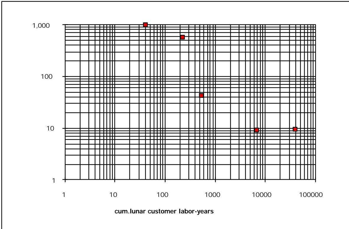
Figure 4-2: Specific cost of lunar labor years performed in leased lunar laboratories for commercial customers as a function of cumulative customer labour-years during the life-cycle ( M 1999 $)
