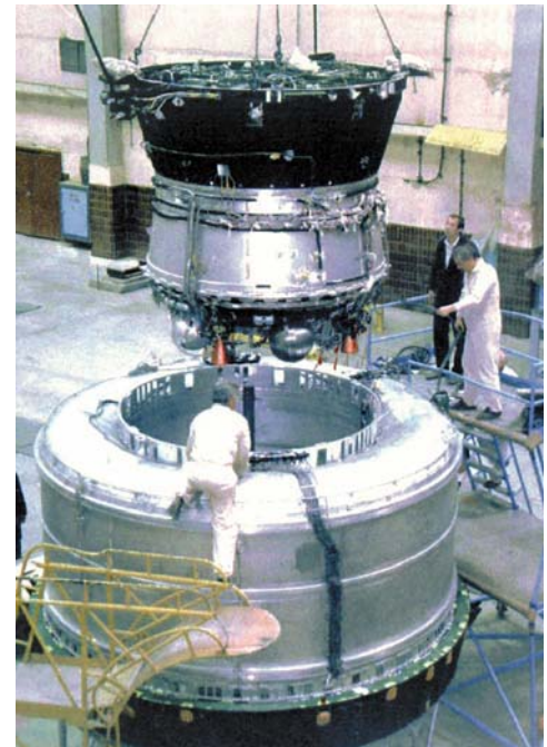
Figure 3.12: Delta IV Heavy Dual-Payload Attach Fitting DPAF-5 (Boeing)
