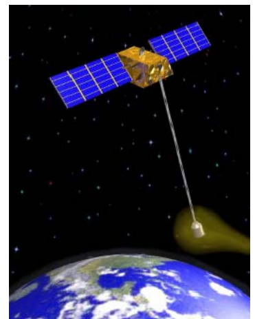
Figure 3.7: De-orbitation of a spacecraft using the Terminator ® electro-dynamic tether (Forward & Hoyt)
