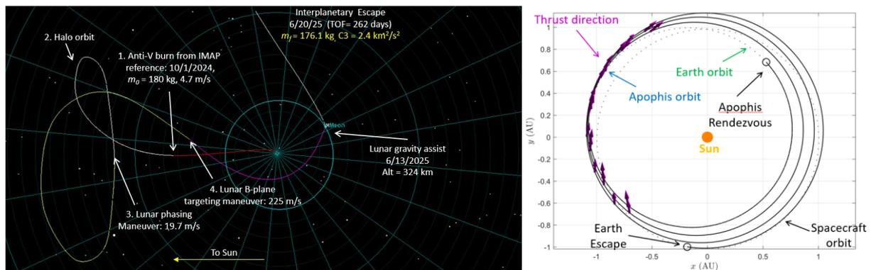
**Figure 3. Low Energy Transfer from IMAP Separation Vector**
