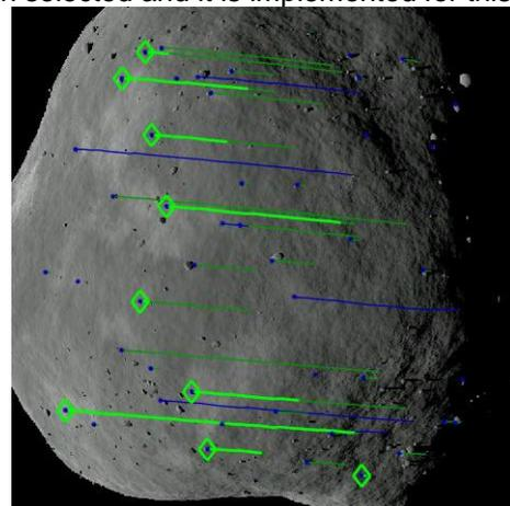
Figure 3: Feature tracking in close fly-by
