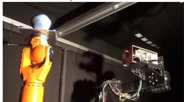
Figure 4: HIL tests in platform-art for AIM (HERA previous activity), currently repeated for HERA scenario
