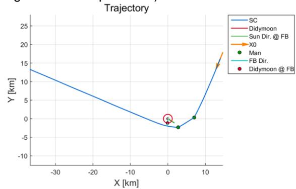
Figure 2: HERA close fly-by with autonomous maneuvers
